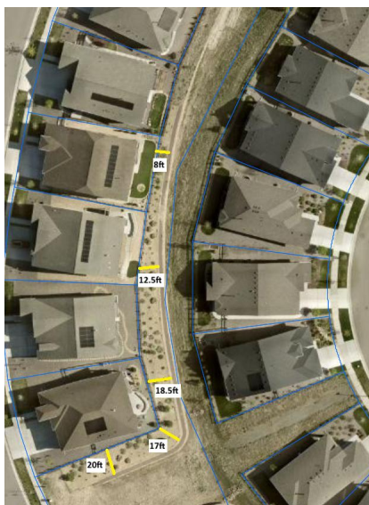
Image: Distance from property fence line to edge of upper wall North side
